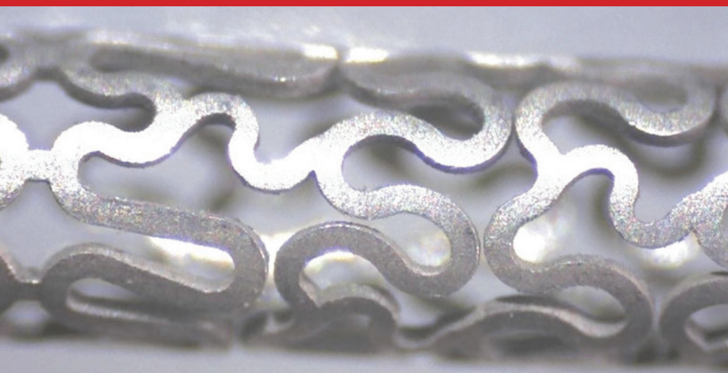
Micro Welding - pulsed fiber laser welding of stainless steel
